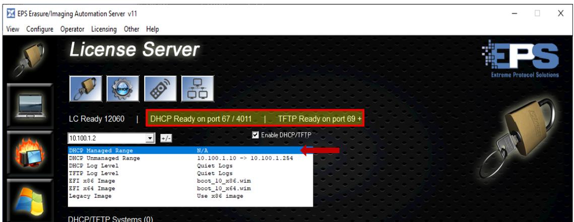
Figure 64 Confirming DHCP Is Configured And Active
