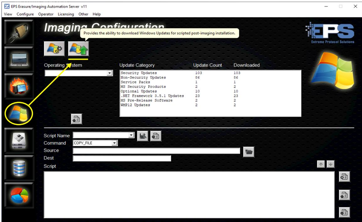
Figure 28 Configuring Windows Updates For Post Installation
